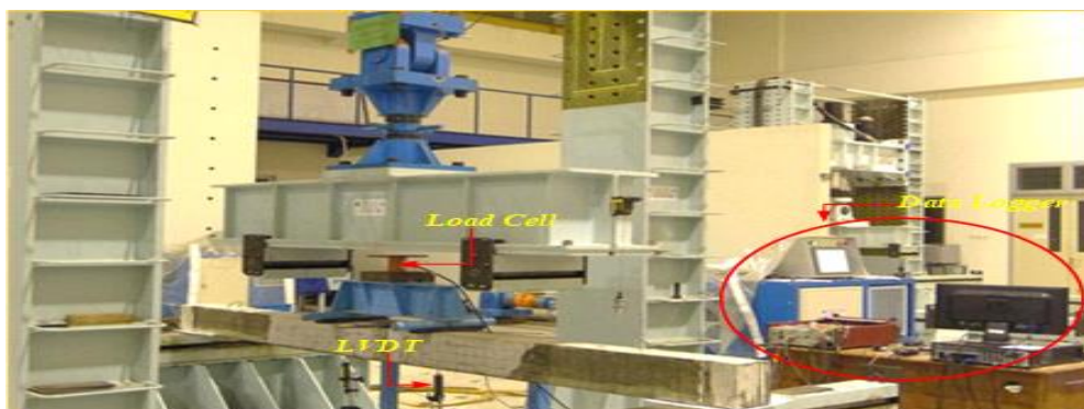
Figure 5. Test specimen setup
