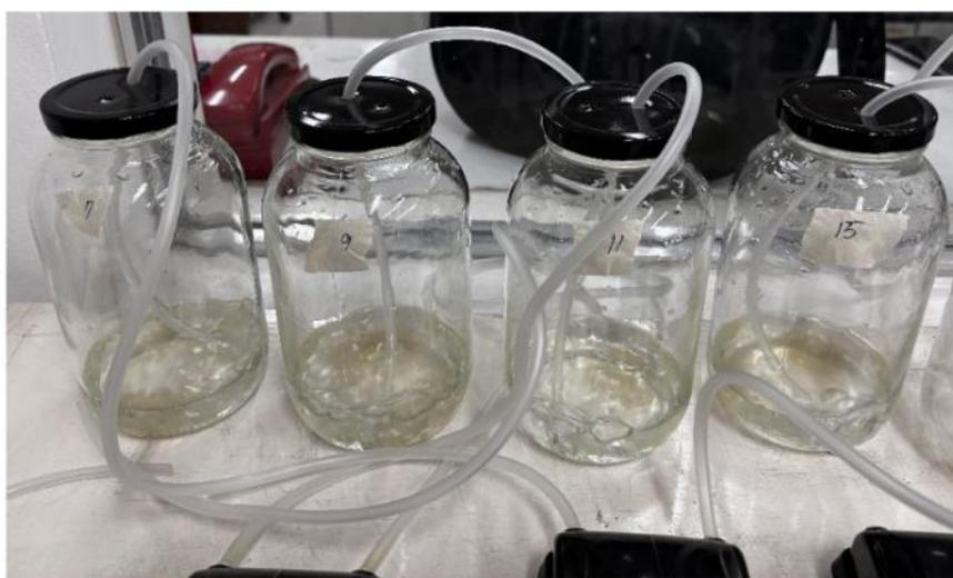
Figure 6. Synthetic wastewater setups with immobilized *S. platensis* beads
