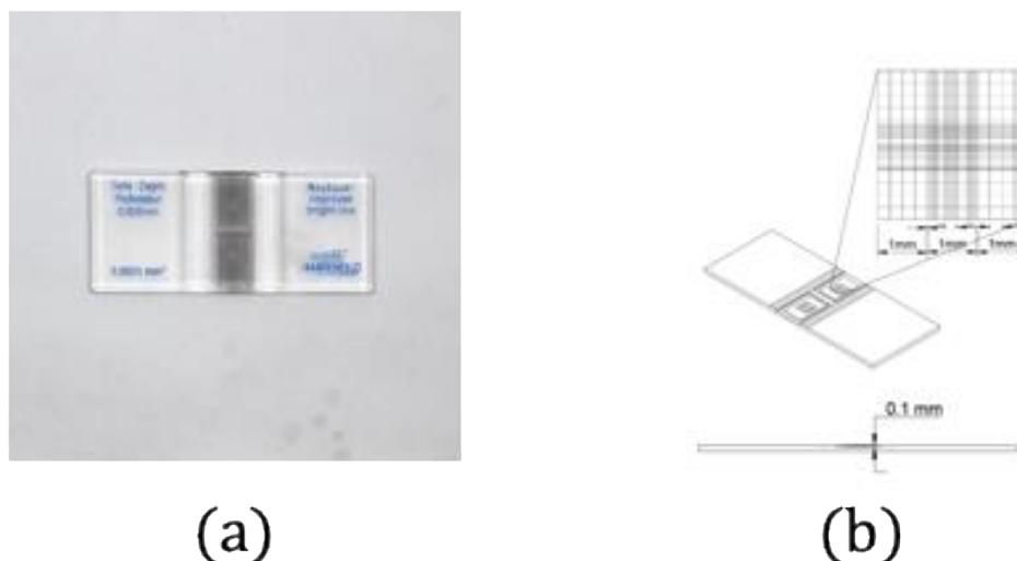
Figure 3. (a) Actual hemocytometer and (b) orthographic and isometric drawings of the hemocytometer
