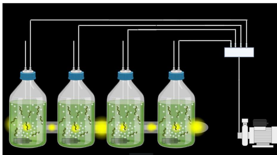
Figure 2. Experimental setup of the *S. platensis* subculture vessels
