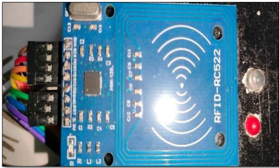
Figure 10. RFID – RC522 for student attendance tracking
